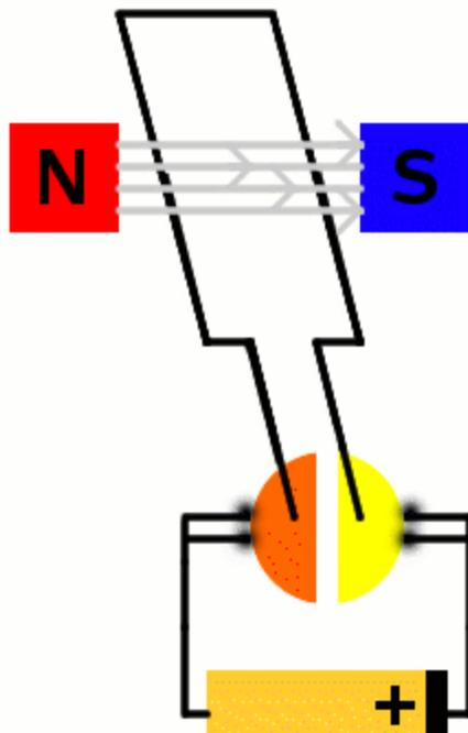
**Figure 2.** This animation shows the direction the loop of wire (the electromagnet) will rotate, based on Fleming's Left Hand Rule for Motors. (ExplainThatStuff.com, 2008.)
