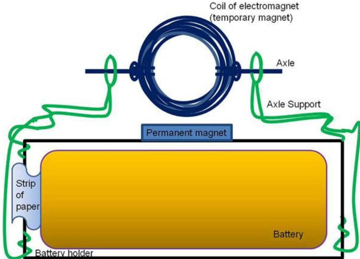
**Figure 5.** This drawing shows how to connect the electromagnet and its axles, the permanent magnet, axle supports, battery, and its paper switch to form a simple electric motor.
